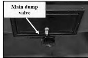
The black tank flush may be used through the gravity dump (by pass valve must be closed).
