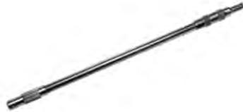
2. Attach flexible shaft to the 1/4" hex fitting on the end of the motor.
