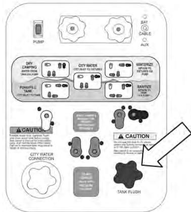
**Sewer Tank Flush Inlet on
