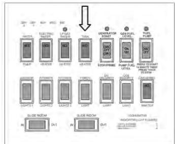
**IMPORTANT:** In order for the 120VAC tank heaters to be in operation, the recreation vehicle MUST be hooked up to shore power or under generator power. If the recreation vehicle is not operating on shore power or generator power, only the +12VDC heaters will operate. This can result in the tanks freezing. The red light on the command center tank switch does not necessarily indicate that ALL heaters are operating; it is a warning that the heater circuit is ON.
