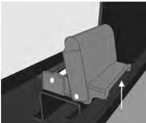
When both latches are released, push out on the window which is hinged at the top. Exit the vehicle.
