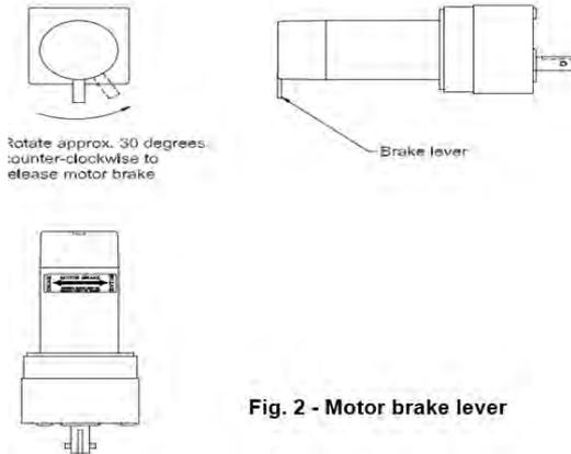
**Fig. 2 - Motor brake lever**
