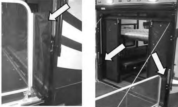
The patio deck comes equipped with mesh end curtains that snap to the door jamb of the rear cargo ramp door (or the side patio door jamb) and to the frame work of the railings. These curtains close off the gap between the railing and the door jamb.
