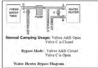
**NOTE:** In the 3-valve bypass diagram, valve D is the fresh water tank shutoff. Valve E is used to introduce RV antifreeze into the lines when winterizing the system and has a clear hose attached to it. See *Winterizing the Plumbing System*. Valves D & E are typically located near the water pump, which may be under a dinette bench, kitchen island, or bed.
